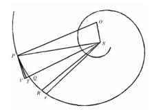
of the arc PQ is a quarter part of the decrement of the arc PR. From which also, if the area PSQ thus may be taken equal to an area QSr, the decrement of the arc PQ will be equal to half the decrement of the linule Rr [see note one below]; and thus the force of resistance and the centripetal force are in turn as the small lines  $\frac{1}{2}Rr$  and TQ, which they produce at
