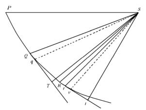
diagram ,as there is a difference in the labeling from the extra diagram here – to the point Q of the arc PQ, generates the decrement TQ, and thus the force of resistance is to the centripetal force as  $\frac{1}{2}Rr$  to TQ, (by Cor. 4, Lem. X), and thus all these may be generally obtained, whatever were the curve PQR, whose properties we have not yet used, nor the centripetal force, the resistance, nor the velocity of the body.]
