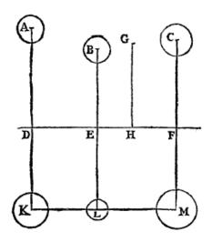
A, B, and C shall be the weights placed in the same part of the plane, the section of which is DF, and the perpendiculars themselves AD, BE, and CF are drawn. Moreover, the centre of gravity of all the weights A, B, and C is G, from which the perpendicular GH is drawn in the same plane. I say that the sum of the products, which are made by the weights taken with their own perpendiculars, is equal to the product of the line GH by the sum of the weights A, B, and C
