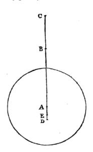
The magnitude, the centre of gravity of which is A, is suspended first and set in motion from the axis B, hence indeed from the axis C; the centre of oscillation in the first case is D, and in the second case it is E. [p.125]. I say that as BA is to CA thus EA is to DA.
