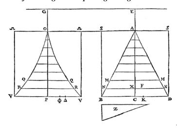
For example, if BD is the greatest of these sections, and it is understood that a line is drawn through B parallel to the axis through E out of the page, *i. e.*, at right angles to the plane which is seen here, and it is necessary to be given the distance of the centre of gravity of the section BD from the given line through B, which is BC; and likewise the subcentre of the wedge, to be cut upon
