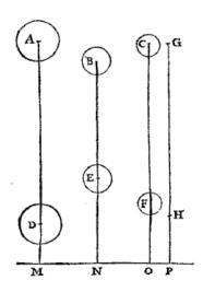
Let the magnitudes be A, B, and C, which descend from A, B, and C to D, E, and F; or from D, E, and F ascend to A, B, and C. The common centre of gravity of all these weights, such as A, B, and C, has the same height as the point G; as indeed that of D, E, and F has the same height as the point H. I say that the sum of the products of the height AD by A, BE by B, and CF by C, is equal to the product of GH by the sum of A, B, and C.
