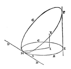
In the added diagram, ABEC is the given figure; the line touching that figure MD; [p. 104] to which truly EF is carried around; moreover the wedge is the solid figure from the planes ABEC and MFG, and from the part of the surface understood to be described by the line EF.
