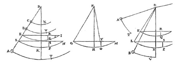
suspended from the axis, which is understood to pass through the point D in a plane, observed at right angles. In which plane the common centre of gravity shall be at E also; for we are not concerned with the different weights. The distance of the point E from the axis, truly the line ED, is called d. Likewise the distance AD of the weight A is e; BD, f; and CD, g. Thus by multiplying the individual weights by the squares of the distances,
