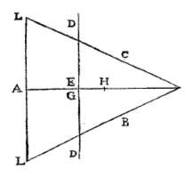
With the same settings as in the preceding proposition; if the given line ED passes through G, the centre of gravity of the figure ABC; then the sum of the squares of the distances of the individual elemental areas, into which the figure is understood to be divided, [p. 109] from the line ED, is equal to the rectangle AGH alone, multiplied by the number of elemental areas.
