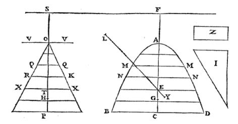
axis is understood to pass through the centre of gravity G, parallel to the axis through F. With the known magnitude divided into the smallest elemental parts, the plane I multiplied by the number of elemental particles is equal to the squares of the distances from the said axis through E. By dividing the plane I by the distance FE, a certain line is produced. I say that line is equal to the interval EG, by which the centre of oscillation lies below the centre of gravity of the magnitude ABCD.
