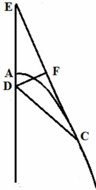
Some line CE shall be a tangent to the parabola ABC at C, meeting the axis AD of the parabola at E,. And with CE bisected at F, the normal FD to the tangent EC crossing the axis at D.
