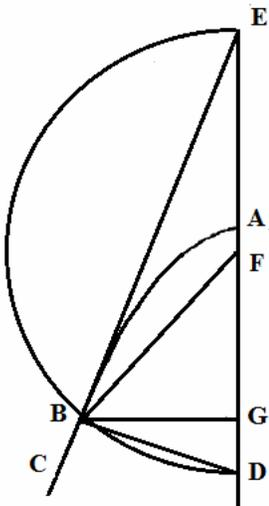
The ordinate line BG [of the latus rectum] shall be put in place : and the normal BD to the tangent EB. Because the angles EBF, BEF are equal from the hypothesis, also the lines FB, FE are equal, and in addition the angle EBD shall be right; if with centre F, a circle shall be described with the radius FE, that will pass through B and D [*elementa*]. Whereby EF, FD shall be equal lines, and thus FA is equal to the fourth part of the latus rectum [§.116 above] . Which was the first part.
