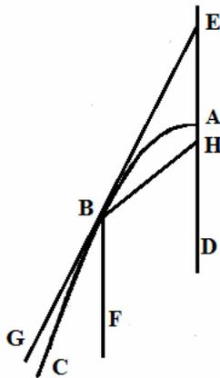
Some right line BE crossing the axis at E shall be a tangent to the parabola ABC, of which AD shall be the axis, and with the line BF dropped from B parallel to the axis, the angle FBG shall become equal to the angle EBH.
