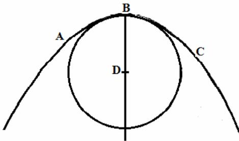
BD shall be the axis of the parabola ABC, it is required to assign on that the point D, so that the centre of the circle described from that point shall be the greatest of these which touch the parabola at only one point, the line DB shall be made equal to half the latus rectum: and with the centre D, the circle shall be described with the radius BD ; I say that to
