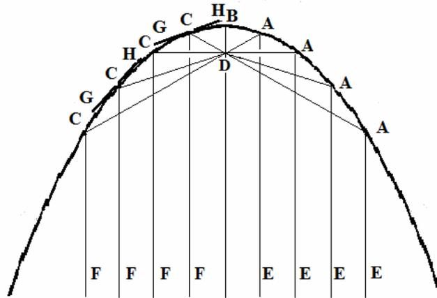
Again we consider the focal point D, because combustion may happen at that point, and the reflected rays gathered together there, may produce an intense heat; since truly the point D (which is determined from the fourth part of the latus rectum from the vertex assumed initially) allows no width: so that the parabolic form shall become the most suitable of all, for the rays from the sun being received and reflected; and produces the effect much more strongly than the remaining figures.
