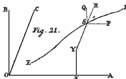
put these things together, we refer the motion to three directrices  $OA$ ,  $OB$  and  $OC$  (Fig. 21) normal between themselves and with the elapse in the time  $t$  the centre of inertia arrives at  $S$ , with the coordinates present  $OX = x$ ,  $XY = y$  and  $YS = z$ . Then the force acting  $V$  is resolved along these three directions, thus the forces arise : along  $SP = P$ ,
