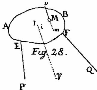
Since the time is assumed as a minimum, the force can be considered meanwhile as constant and acting in the same direction. Therefore let the mass of the rigid body be equal to  $M$ , to this is applied the force equal to  $V$ , the direction of this  $IV$  passes through the centre of inertia  $I$  (Fig. 28). Hence the point  $I$  will begin to move forwards in this direction  $IV$  and the whole body likewise gains a similar progressive motion.
