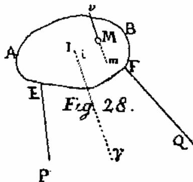
At a given time the body is acted on by forces  $EP$  and  $FQ$  (Fig. 28), for which the equivalent force  $IV = V$  passing through the centre of inertia  $I$ , which, if the mass of the body should be equal to  $M$ , will produce the same effect in the whole body; and on some element of this mass  $M$ , the mass of which is  $dM$ , the force produced is then
