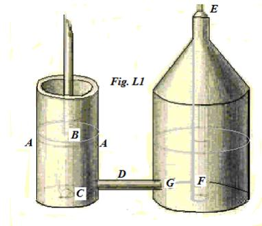
In this machine a large part of the *work done* is lost in the transition of water by the pipe  $D$ , and that loss will be greater there, when this tube is narrower: therefore it may be made wider or also several tubes may be constructed transmitting water: but in the present case this annotation is of the greatest concern, because a much greater loss arises from the narrow pipe  $D$ , than from other machines ; for make the cross-section of this
