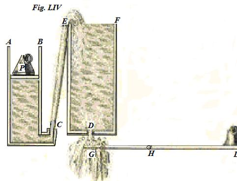
machine a simple lever is described turning around  $H$ , by putting such a lever continually one after another to be present before the opening  $D$ , which may accept the water, and by its other extremity may draw up water, and raise it to the same given height.
