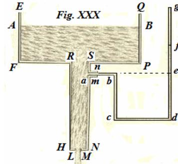
$FA = \frac{nn}{mm - nn} a$ , with  $\frac{n}{m}$  denoting the ratio between the lower opening *LM* and the upper *RS*, and *a* the vertical height of the latter opening above the former.
