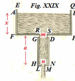
The water may begin to flow out from each vessel, but put to flow from that upper one constantly with the velocity that the surface of the water has in the cylinder placed below. Thus it appears to satisfy the first condition of affusion. Now truly we will investigate the phenomena of this motion, to see whether they will agree with the preceding.
