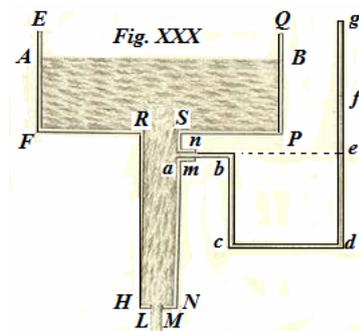
experiment the surface of the water shall remain constantly at the point *e*; and you will see towards this to be required, that from the beginning the surface of the water shall be approximately at the bottom *FP*, then, so that it is raised continually, and at last so that after a time even if infinite it will at no point pass beyond the height
